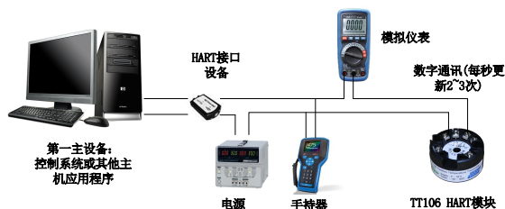
Figure 3.14~20mA compatible mode
