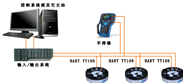
Figure 3.2 HART Networking mode
